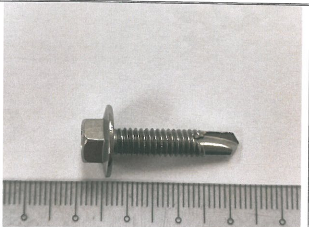
Appearance of NSSC 550 IND HEX WASHER HEAD DRILLING SCREW CSD(#12x1")-1 after 6000 hours salt spray test
