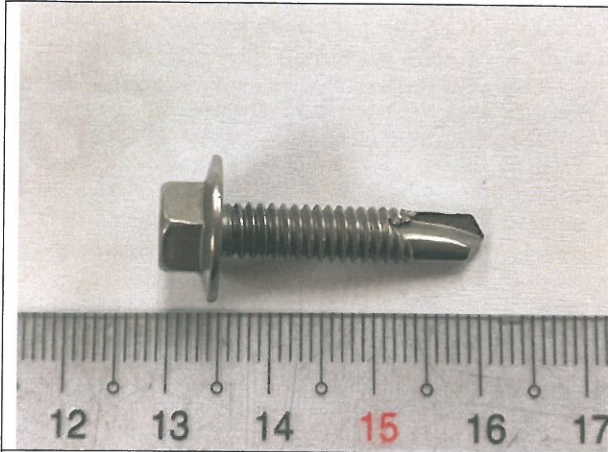
Appearance of NSSC 550 IND HEX WASHER HEAD DRILLING SCREW CSD(#12x1")-1 after 7000 hours salt spray test
