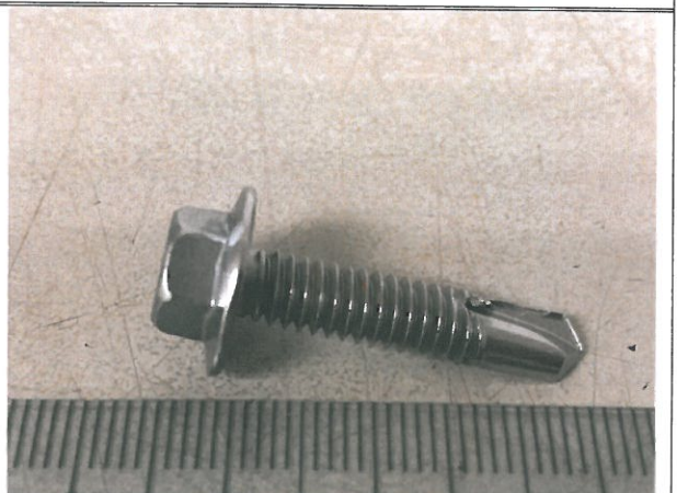
Appearance of NSSC 550 IND HEX WASHER HEAD DRILLING SCREW CSD(#12x1")-1 after 2000 hours salt spray test
