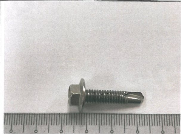
Appearance of NSSC 550 IND HEX WASHER HEAD DRILLING SCREW CSD(#12x1")-1 after 5000 hours salt spray test
