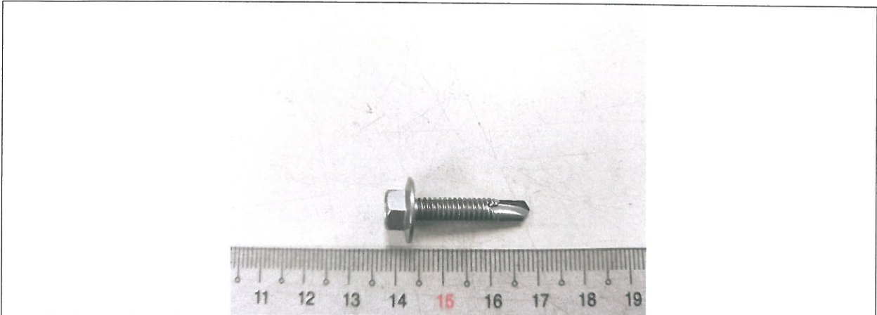
Appearance of NSSC 550 IND HEX WASHER HEAD DRILLING SCREW CSD(#12x1")-1 before 8000 hours salt spray test
